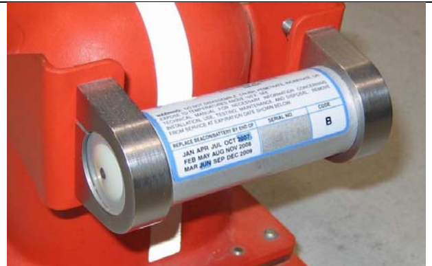
Figure 2b. ULB mounted on the side of an FDR shown together with the expiration date (June, 2007)
