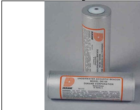
Figure 2a. Detailed view of a ULB on with the positive node shown on the vertical unit.
