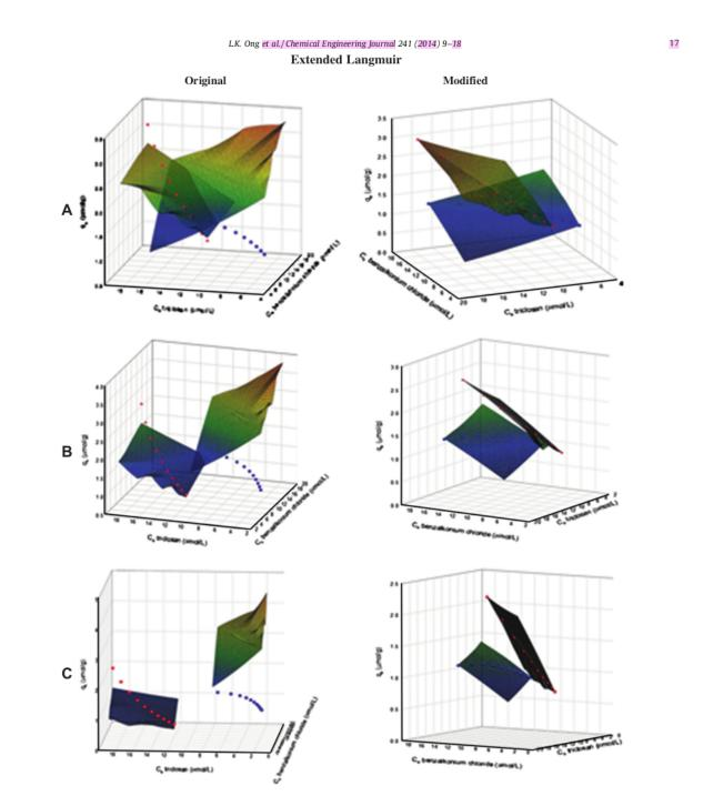
Fig. 3. The aptness of original and modified extended Langmuir models against experimental binary adsorption data of benzalkonium chloride (BAC-•) and triclosan (TCS-•) at 303.15 K onto S-bentonite using. (A) C<sub>o</sub> benzalkonium chloride = 20 µmol/L, C<sub>o</sub>triclosan = 20 µmol/L, (B) C<sub>o</sub> benzalkonium chloride = 15 µmol/L, C<sub>o</sub> triclosan = 20 µmol/L, (C) C<sub>o</sub> benzalkonium chloride = 10 µmol/L, C<sub>o</sub> triclosan = 20 µmol/L.
