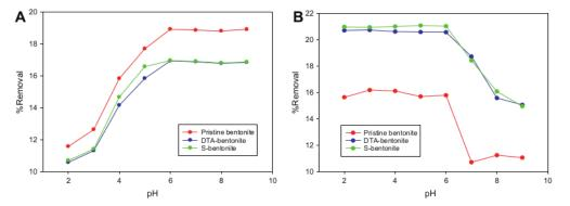
Fig. 1. Effect of the pH on the adsorption of benzalkonium chloride (A) and triclosan (B) onto the pristine bentonite, DTA-bentonite and S-bentonite (m adsorbent = 0.1 g, T = 303.15 K, t = 1 h).
