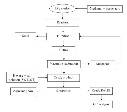
Fig. 2. Flowchart of biodiesel production from dried sludge.
