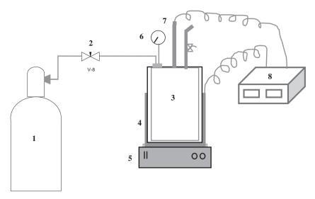
Fig. 1. Layout of equipments for in situ transesterification of activated sludge. [1] Nitrogen cylinder, [2] needle valve, [3] reactor, [4] heater, [5] magnetic stirrer, [6] pressure gauge, [7] thermo couple, [8] controller.
