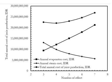
Figure 3. The relationship between the number of effects and the evaporator cost, steam cost, and total annual cost for the production of 125,000 kg/h of syrup
