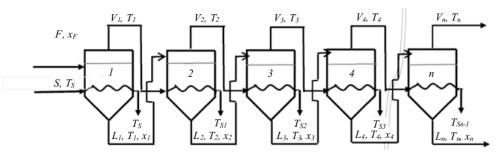
Figure 2. Multiple effect evaporator with number of effects n forward feed type
