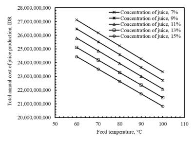
**Figure 6.** The relationship between feed temperature and the total annual juice production cost for various juice concentrations in the feed in a quadruple effect evaporator system.
