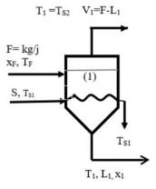
Figure 1. Single effect evaporator (Redrawn from [3])
