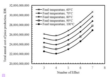
Figure 4. Effect of the number of effects on the annual total juice production cost for various feed temperatures at a feed rate of 125,000 kg/h and a feed concentration of 11%.
