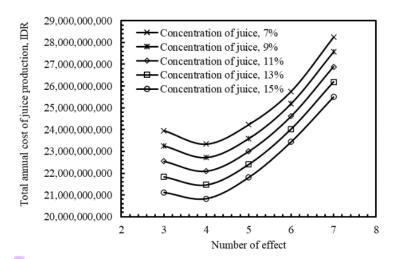
Figure 5. Effect of number of effects on total annual juice production cost for various feed juice concentrations at 100°C feed temperature
