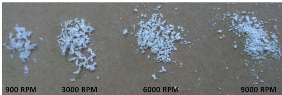
Fig.6 Chip formation on various RPM (Feed rate= 100 mm/ min, HSS flat endmill \varnothing 2mm)
