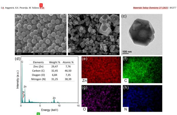
5 Fig. 1. SEM images of (a) PS and (b) HZIF-8, (c) TEM image of HZIF-8, (d) EDX of HZIF-8, and (e-h) the elemental mapping of HZIF-8. EDX, energy-dispersive X-ray spectroscopy; HZIF, hollow zeolitic-imidazolate framework; SEM, scanning electron microscopy.
