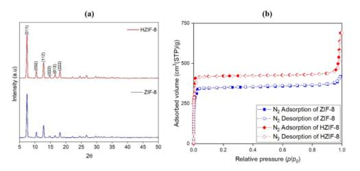
Fig. 2. (a) The XRD analysis and (b) N<sub>2</sub> adsorption/desorption profile of HZIF-8 and ZIF-8. HZIF, hollow zeolitic-imidazolate framework; XRD, X-ray powder diffraction; ZIF, zeolitic-imidazolate framework.
