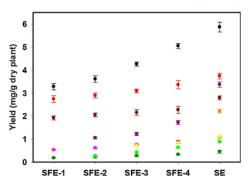
Fig. 2. Extraction yields of several phenolic compounds ( ● quercetin; ● gallic acid; ● p-coumaric acid; ● rutin; ● luteolin; ● kaempferol; ● ferulic acid; ● (+)-catechin; and ● caffeic acid) obtained from soxhlet extraction and SC-CO<sub>2</sub> extraction at a pressure of 22.5 MPa and various temperatures (SFE-1/313.15 K; SFE-2/323.15 K; SFE-3/333.15 K; and SFE-4/343.15 K).
