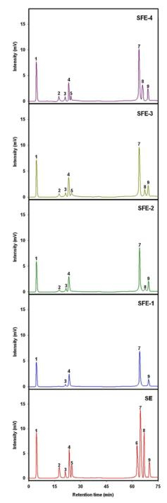
Fig. 1. HPLC chromatograms of antioxidant extracts obtained from soxhlet extraction and SC-Constant extraction. The identified compounds are designated by numbers as follows: gallic acid (1); (+)-catechin (2); caffeic acid (3); p-coumaric acid (4); ferulic acid (5); rutin (6); quercetin (7); luteolin (8) and kaempferol (9).
