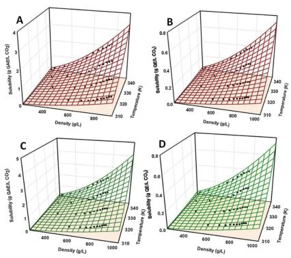
Fig. 4. 3D-fitting of Chrastil (A-B) and Del Valle-Aguilera (C-D) models on the experimental solubilities of polyphenols (g GAE/L CO2) and flavonoids (g QE/L CO2).
