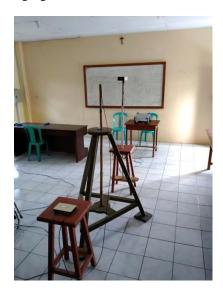
Figure 4. Radiation Pattern Measurement Configuration
