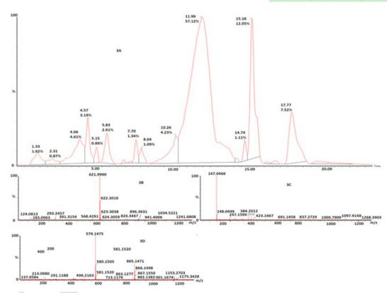
Fig. 3. LCMS of *C. burmannii* extract (3A) chromatogram peak of UPLC, mass fragments ES positive mode at Rt; (3B) 11.96 min (57.12%) with m/z 621.2999; (3C) 7.7 min (1.34%) with m/z 147.0466; (3D) 4.06 min (4.61%) with m/z 579.1475.
