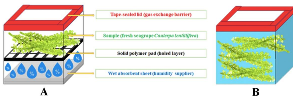
Figure 1. Packaging prototype for the oxidative stress environment (A) storage without seawater (B) storage within seawater.
