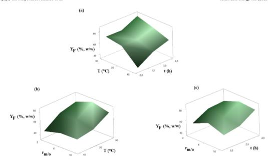
Fig. 4. The FAME yield  $Y_F$  (%, w/w) at various (a) T and t, (b) T and  $r_{m/o}$  and (c) t and  $r_{m/o}$ .
