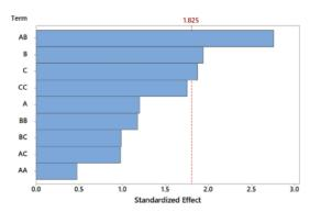
**Fig. 5.** Pareto chart of the standardized effect for the biodiesel preparation with Fe/DS-HMS-NH<sub>2</sub>, using  $Y_F$  as the response at a 95% confidence interval where A=T, B=t,  $C=r_{m/\alpha}$ .
