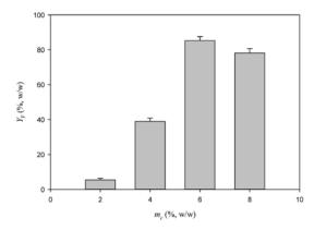
Fig. 3. The yield of FAME at various Fe/DS-HMS-NH $_2$  loadings with the reaction condition of T=60 °C, t=4.5 h and  $r_{\rm m/o}=10$ :1.
