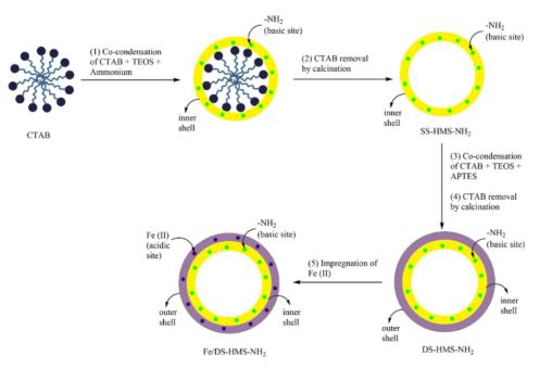
Fig. 1. The mechanism scheme of Fe/DS-HMS-NH2 fabrication.
