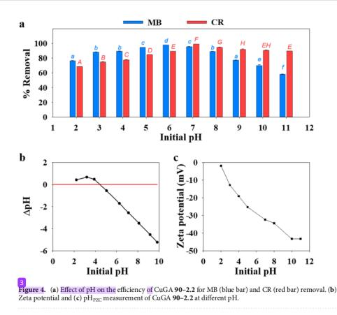
The negative surface charge is also confirmed from the zeta potential value (Fig. 4c). At pH 6, CuGA **90–2.2** has a surface charge that is opposite from the cationic MB, suggesting that their interactions was driven by electrostatic forces<sup>31</sup>. Meanwhile, binding mechanisms such as  $\pi$ - $\pi$  stacking<sup>32</sup>, might be the contributing force for the interaction of CuGA **90–2.2** and CR since both are negatively charged at pH 7.
