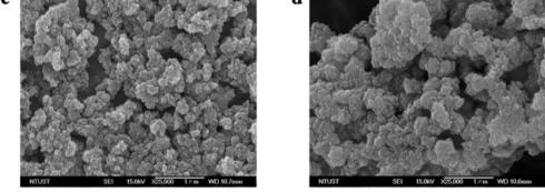
**Figure 7.** Characterization of post-adsorption CuGA **90–2.2**. (a) FTIR spectra of MB-loaded CuGA (MB@ CuGA) and CR-loaded CuGA (CR@CuGA). (b) XRD crystallography of CuGA after 5 adsorption–desorption cycles. (c) and (d) SEM image of MB@CuGA (c) and CR@CuGA (d).
