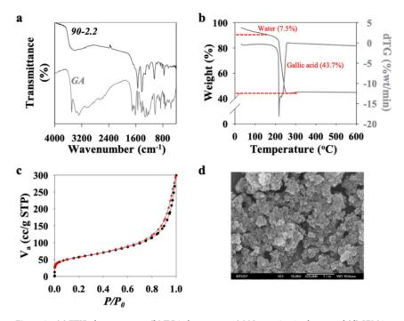
**Figure 3.** (a) FTIR chromatogram, (b) TGA thermogram, (c) N<sub>2</sub> sorption isotherm, and (d) SEM image of CuGA **90–2.2**.
