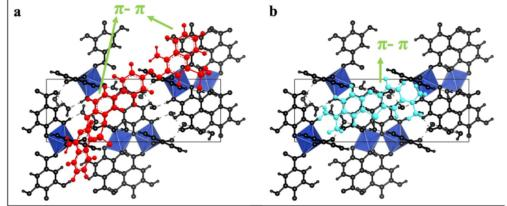
Figure 6. Illustration of possible mechanism of (a) CR and (b) MB adsorption onto CuGA 90-2.2.
