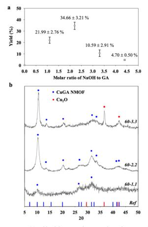
**Figure 1.** (a) Yield and (b) PXRD of CuGA synthesized at 60 °C with different molar ratio of NaOH to GA. The reference XRD pattern was adopted from reported data by Sharma et al.<sup>19</sup>.
