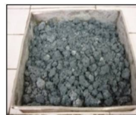
Figure 3. Chromium waste after firing at 110^\circ\text{C} for 4.5 hours.
