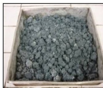
Figure 3. Chromium waste after firing at 110\text{ }^\circ\text{C} for 4.5 hours.
