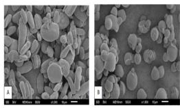
Figure 2. The particle shape of starch using SEM: (A) banana peel starch, (B) cassava starch, with the magnitude of 1000x.
