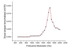
Figure 4.4 Resonance Curve laser lines for ammonia gas
