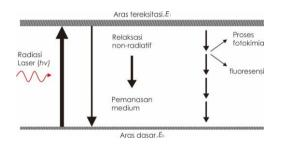
Figure 2.1 Some Type Process Occurred On Ground State Towards Molecular Basis After Radiation Absorbing Laser (*hv*)
