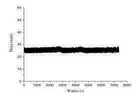
Figure 4.2. CO<sub>2</sub> laser power stability on the line 10R14
