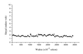
Figure 4.5. Signal noise photoacoustic cell
