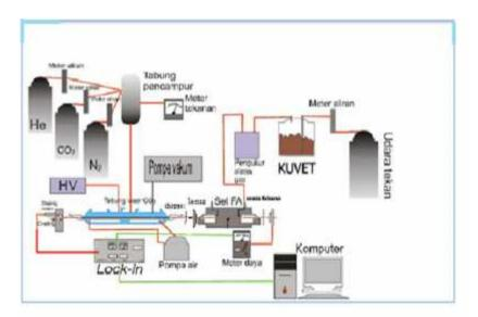
Figure 2.1 Laser CO2 photoelectric spectroscopy kit
