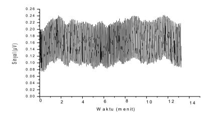
Figure 3.1 CO<sub>2</sub> laser noise
