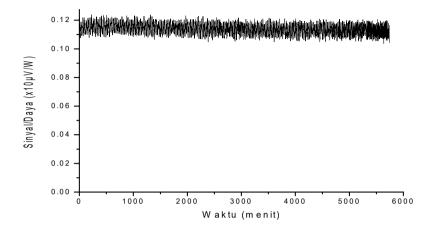
Figure 3.2 CO<sub>2</sub> laser background signal.
