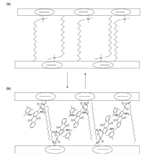
Figure 8. (a) The formation of organobentonite and (b) the interaction between the negatively charged adsorbent surface and the positively charged adsorbate.
