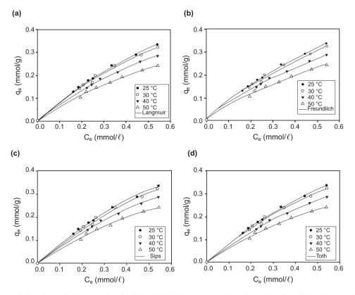
**Figure 4.** Experimental adsorption data for Acid Blue 129 dye onto raw bentonite and the fits of the (a) Langmuir, (b) Freundlich, (c) Sips and (d) Toth model equations.
