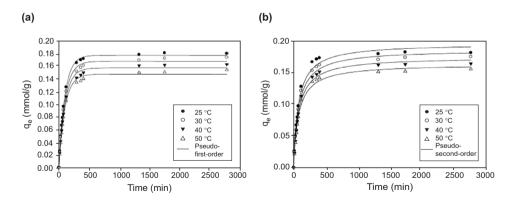
Figure 9. Adsorption kinetics of Acid Blue 129 dye onto raw bentonite and the application of (a) the pseudo-first-order model and (b) the pseudo-second-order model to the experimental data.
