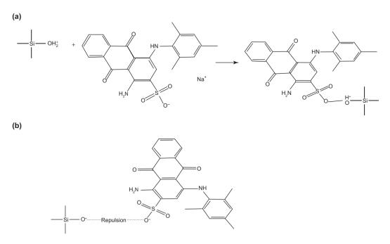
**Figure 7.** (a) Interaction between the protonated silanol groups in bentonite and the negatively charged Acid Blue 129 ions. (b) Ionic repulsion between the negatively charged adsorbent surface and the anionic dye molecules.
