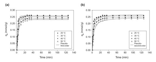
Figure 10. Adsorption kinetics of Acid Blue dye 129 onto organobentonite and the application of (a) the pseudo-first-order model and (b) the pseudo-second-order model to the experimental data.
