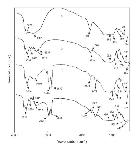
Figure 1. FT-IR spectra for bentonite samples: (a) raw bentonite; (b) dye-loaded raw bentonite; (c) organobentonite; and (d) dye-loaded organobentonite.
