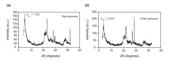
Figure 2. XRD patterns for (a) raw bentonite and (b) organobentonite.
