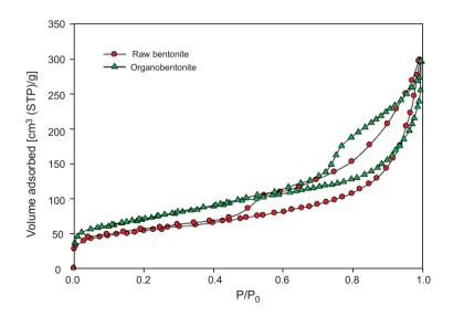
Figure 3. Nitrogen sorption isotherms for raw bentonite and organobentonite.
