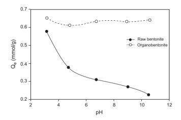
Figure 6. Effect of the solution pH on the adsorption performance of raw bentonite and organobentonite.
