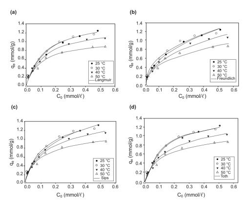
**Figure 5.** Experimental adsorption data for Acid Blue 129 dye onto organobentonite and the fits of the (a) Langmuir, (b) Freundlich, (c) Sips and (d) Toth model equations.
