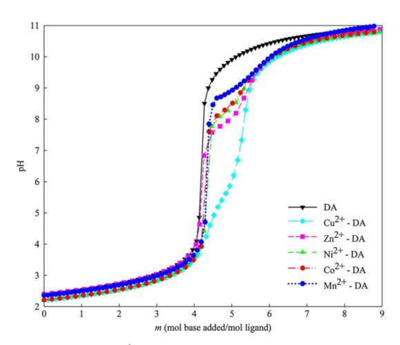
Fig. 2 Titration curve for the M<sup>2+</sup>-DA system at a metal to ligand ratio of 1:2.5
