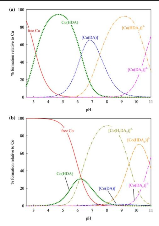
Fig. 3 Speciation diagram of binary a Cu<sup>2+</sup>-DA and b Co<sup>2+</sup>-DA at metal to ligand ratio of 1:2.5
