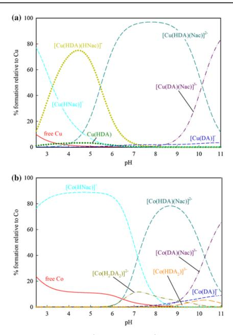
Fig. 5 Speciation diagram of ternary a Cu<sup>2+</sup>-DA-Nac and b Co<sup>2+</sup>-DA-Nac at metal to ligand ratio of 1:1:1
