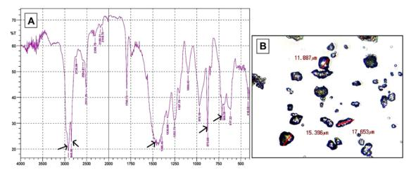
Figure 1 (A) Fourier-transform infrared spectroscopy examination. (B) Microscope observation of low-density polyethylene microplastic particles.
