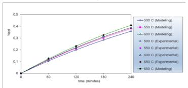
Figure 4. Yield biochar for pyrolisis time if katalis of Mo/bentonit
