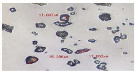
**Figure 1.** Microscopic picture of polyethylene particles that have been filtered to a size less than 20  $\mu$ m using the FCT Z100 miller machine.
