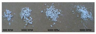
Fig.6 Chip formation on various RPM (Feed rate= 100 mm/ min, HSS flat endmill Ø2mm)
