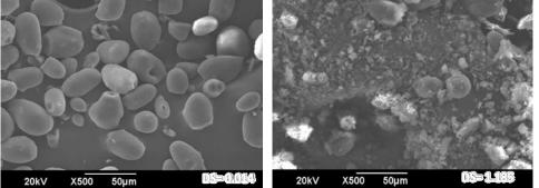
Figure 3. Scanning electron micrograph of native and sago starch acetate
