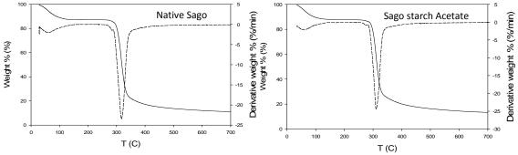
Figure 2. Thermogravimetric curves of native sago starch and sago starch acetate. Weight loss curve (-). Derivative of weight loss (--)
