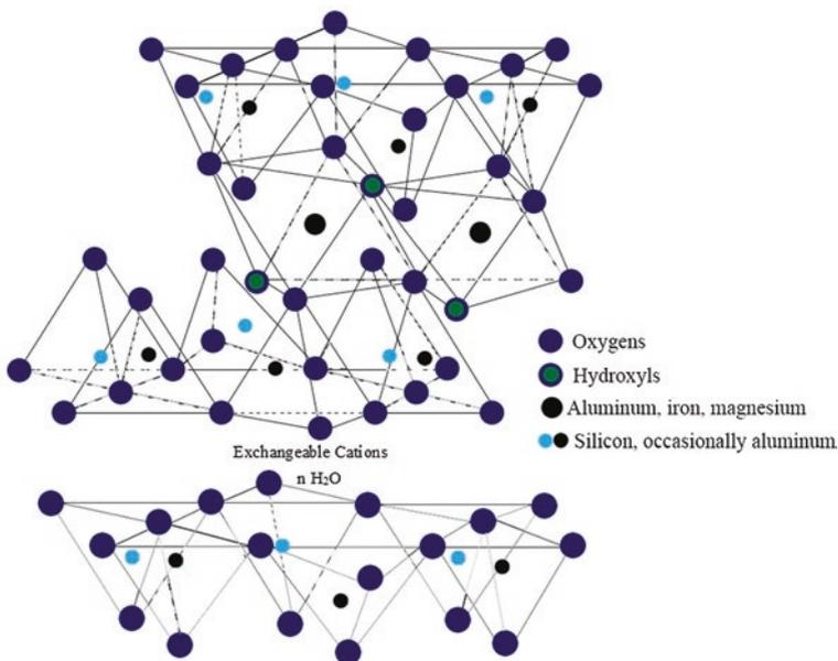
Fig. 2.2 The structure of smectite clay (redrawn based on Murray 2007)
