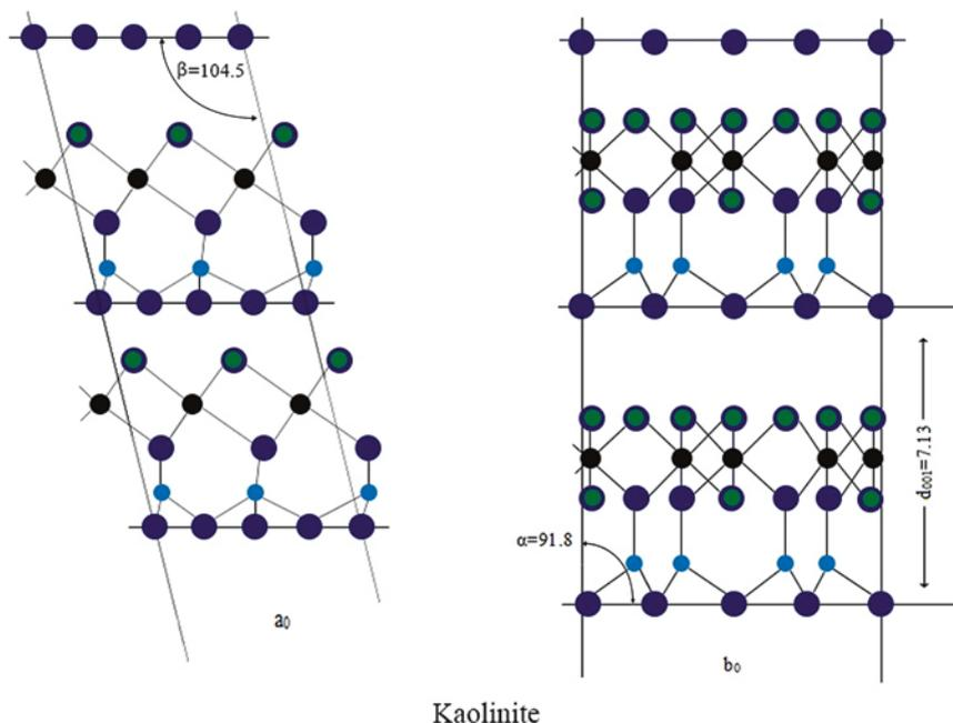
**Fig. 2.1** Schematic diagram of kaolinite structure (redrawn based on Murray 2007)
