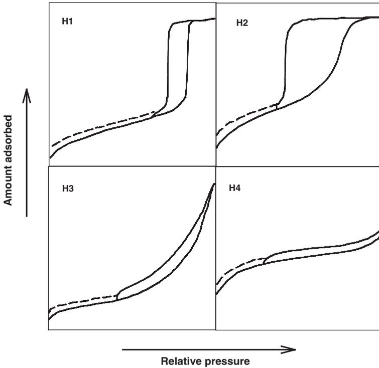
Fig. 5.2 Relation between the hysteresis of sorption isotherm and the pore shape (Allothman 2012)
