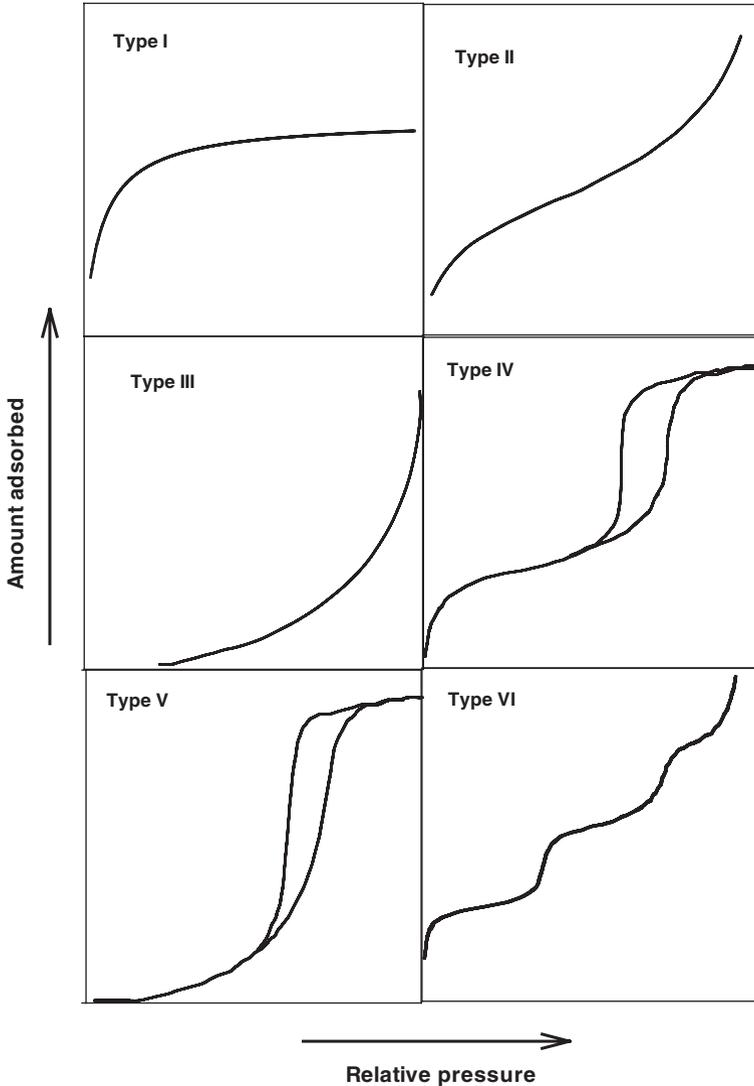
**Fig. 5.1** The IUPAC classification of adsorption isotherm (Allothman 2012)
