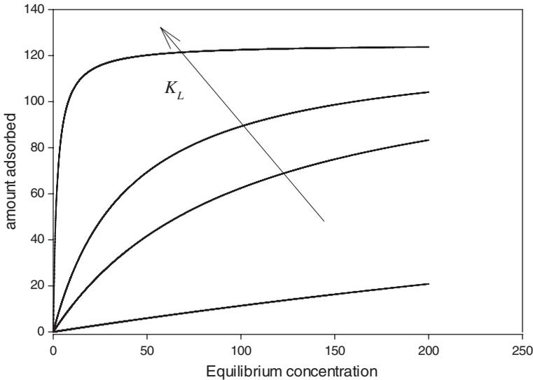
**Fig. 4.1** The effect of the value of parameter  $K_L$  on the amount of solute adsorbed by the adsorbent
