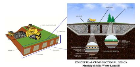
Figure 26.2 Schematic diagram of a landfill design.
