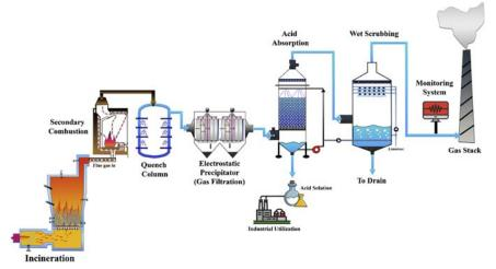
Figure 26.3 The overview of an incineration system fully equipped with the APCE.
