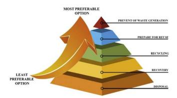
Figure 26.5 The five-stage waste management hierarchy in the European Waste Framework Directive.
