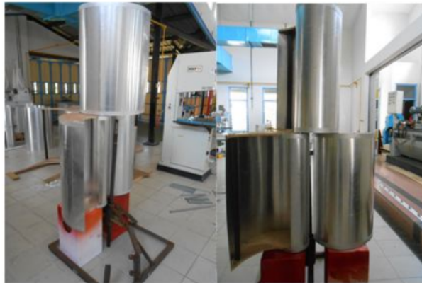
Figure 4. The design of shafts and blades for vertical axis wind turbine.
