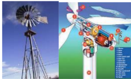
Figure 1. Horizontal axis wind turbine and its parts (www.wilsonms.pbworks.com)
