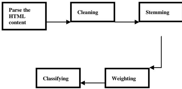
Fig 1. The complete block diagram of the webpages classification
