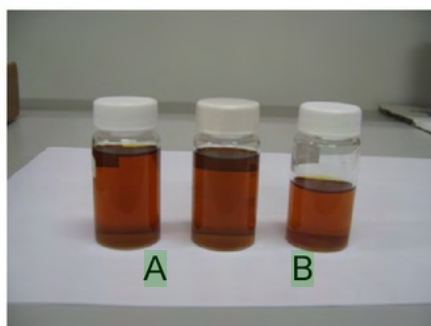
Fig. 8 \text{TiO}_2 suspensions with 10 mL of TEA and different volume of LA: (A) 18 and (B) 24 mL
