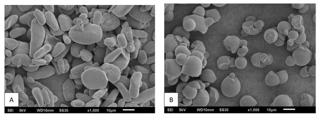
Figure 2. The particle shape of starch using SEM: (A) banana peel starch, (B) cassava starch, with the magnitude of 1000×.
