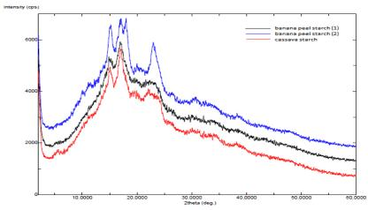
Figure 4. XRD patterns of banana peel and cassava starches.
