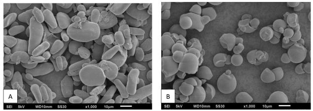
Figure 2. The particle shape of starch using SEM: (A) banana peel starch, (B) cassava starch, with the magnitude of  $1000 \times$ .
