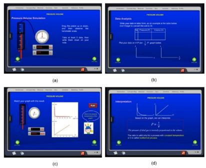
Figure 2 Simulation of *P-V* relationship. The simulation contains some activities such as (a) data collecting, (b) data analysis, (c) confirmation of result through automatic simulation, and (d) interpretation of result.
