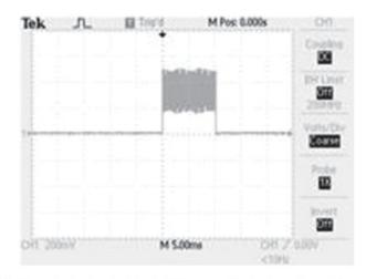
Fig. 32.7 Ultrasonic signal emitted by the ULB captured by the ultrasonic transducer
