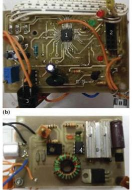
Figure 32.6a shows the top circuit board of the tester with marking (1, 2, 3) of the microcontroller, connector to the LCD module, and buzzer. Figure 32.6b shows marking (4, 5) the ultrasonic amplifier and the ultrasonic transducer itself.
