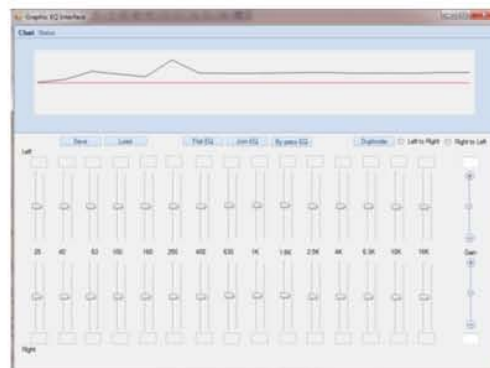
Fig. 3(b): Digital control interface of the digital equalizer.
