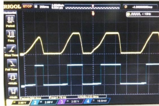
Fig. 10. Pulses waveform vs comparator output waveform
