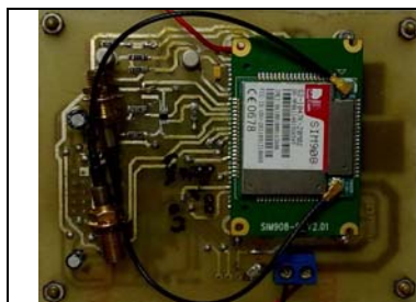
Figure-5a. Top side of the GPS vehicle tracking with the SIM908 module shown on top of it.
