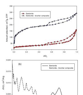
Fig. 1. (a) Nitrogen adsorption—desorption isotherms of bentonite and bentonite — biochar nanocomposite, and (b) Density functional theory pore size distribution of bentonite and bentonite—biochar nanocomposite.
