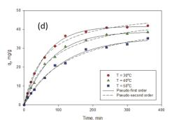
Fig. 7. Adsorption kinetic and plots of pseudo-first and pseudo-second order models (a) Cu(II) onto bentonite, (b) Cu(II) onto bentonite – biochar composite, (c) Pb(II) onto bentonite, and (d) Pb(II) onto bentonite – biochar nanocomposite.
