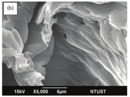
Fig. 4. SEM images of (a) bentonite and (b) bentonite - biochar nanocomposite.
