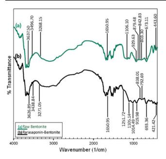
Fig. 2 FTIR spectra of natural bentonite and rarasaponin-bentonite
