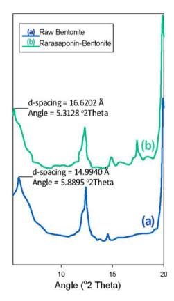
Fig. 3 XRD results of natural bentonite and rarasaponin–bentonite Adsorption study
